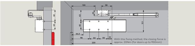
(Example refers to left-hand [ISO 6] door; mirror image applies to right-hand [ISO 5] door). Parallel-arm bracket (accessory) necessary
